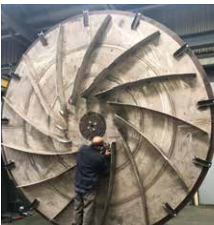
Converter gas fan with 3.9 m diameter, made from high-end stainless steel, operated at 230 m/s with continuous water injection.
