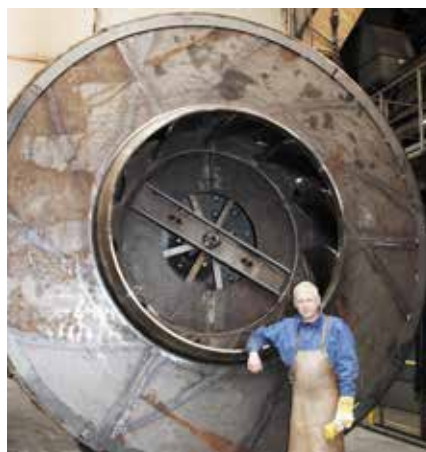
Fan for sinter dedusting, 4.0 m impeller diameter, double inlet and equipped with carbide wear protection. Shaft power 7.500 KW.
